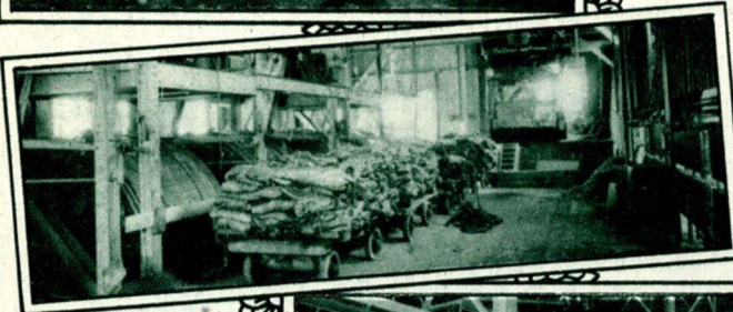
Dry hides are soaked in these drums to make them soft and workable.
