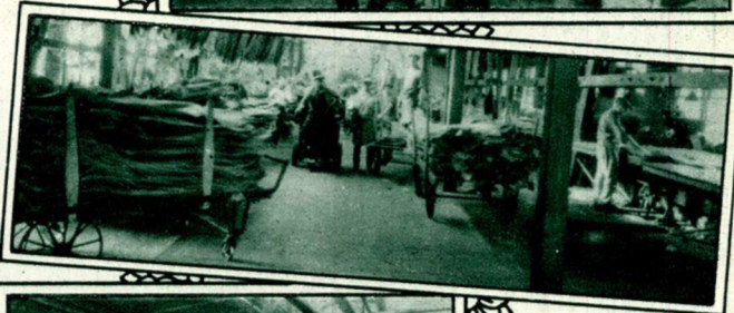
After the leather is tanned and dried it is sometimes wavy and slightly wrinkled. These machines called the "rollers," smooth the leather and put on a shiny surface.
